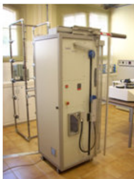
Fig. 2. Dynamometry gradient constant elongation installation
